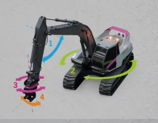
**Solution:** Two movement axes are standard with excavators.
